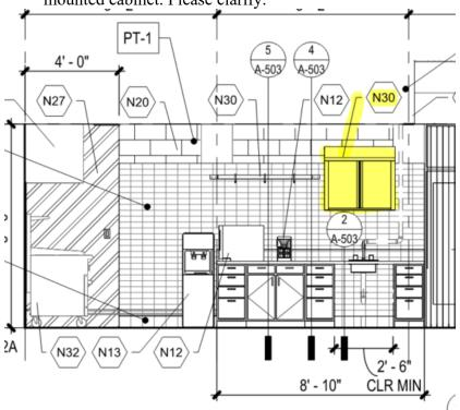
**RESPONSE:** Follow equipment schedule – Sheet A-604 for clarification between wall mounted cabinet and pot rack. Highlighted element is wall mounted cabinet.
