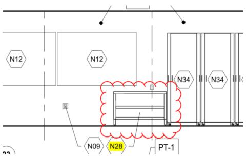
**RESPONSE**: Commercial Grade premanufactured SST dish cabinet. Provide 1 as shown in plan and elevation.
